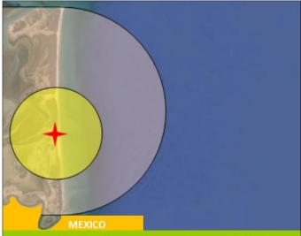
**Figure 1** - The yellow blast zone (notional) around the launch pad is established through Explosive Safety Quantity Distance (ESQD) calculations, taking into account the worst-case explosive potential of a fully fueled rocket sitting on the launch pad. The larger half-circle is a water closure area that would extend from the south jetty of the Brazos Santiago Pass, 7.5 miles down to the Rio Grande U.S./Mexico border.
